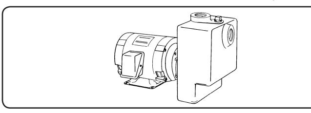
**CASING** - Casing is close grain iron of 30,000 psi minimum tensile strength. Back pull-out design eliminates the need to disturb piping should the pump ever require service - the casing stays in the line.
