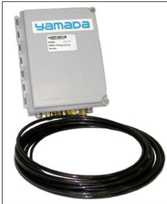
The Yamada LLC-2 Liquid Level Controller is a totally pneumatic system designed to automatically start and stop Yamada Air-Operated Double Diaphragm Pumps when the liquid level within a tank, sump, etc. reach predetermined levels.
