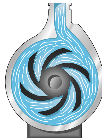
STAN-COR Concentric Casing Pump showing smooth flow pattern
