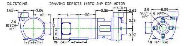
ALL DIMENSIONS IN INCHES. DRAWING REPRESENTS APPROXIMATE PUMP DIMENSIONS. AUTOCAD DRAWING TO SCALE AVAILABLE FROM FACTORY.
