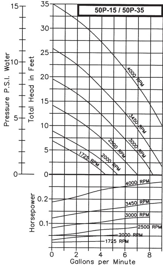
used at the beginning of the suction line and all air is bled from the suction line and pump by careful manual priming, these pumps will lift liquid on the suction side up to 15 ft. Such a system is only as positive as the ability of the foot valve to seal and keep the suction line and pump full of liquid. If the foot valve should leak, the pump will not prime.
