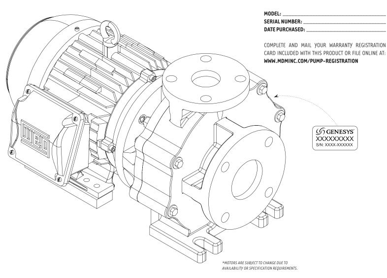
**TYPE:** END-SUCTION CENTRIFUGAL **SEAL OPTIONS:** IMPENATRA® II NON-METALIC MECHANICAL SEAL:
