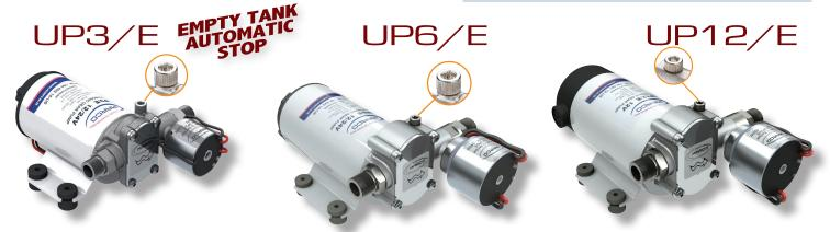
Self-priming automatic electric pumps with helical PTFE gears, integrated check valve and electronic control. Nickel-plated brass body and stainless steel shaft. Control panel available.
