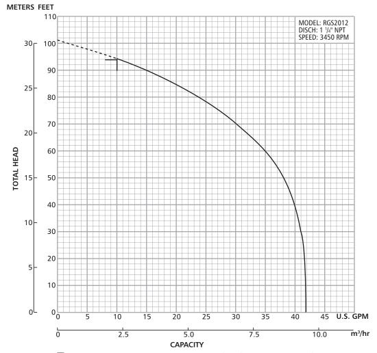
= A 1<sup>1</sup>/<sub>4</sub>" minimum discharge pipe requires a minimum flow of 10 gpm to maintain a 2 ft./sec. scouring velocity. Flows less than 10 gpm will allow solids to settle in the pipe.
