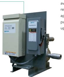
Specifically designed as a compact, easy to install and maintain package for applications where sufficient main pressure is not available or elevation is a problem. Typical installations include residences, apartment buildings, condominiums and light commercial applications. The AquaBoost VS is available in both one and two pump packages. Simplex capacities range from 20 to 110 GPM at a boost of up to 55 psig. Duplex capacities are up to 220 GPM.
