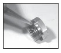
4) Remove the o-ring (31). Inspect all parts for wear and replace as necessary. Apply one drop of loctite 243 to the valve plugs (32) and tighten to 125 ft. lbs.
