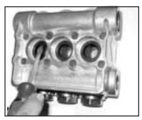
7) Remove the pressure rings (24) and v-sleeves (23 - Note: P422 & P423 pumps have a support ring) from the valve casing (26).
