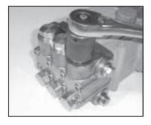
1) With a socket wrench, remove the three discharge valve plugs and three inlet valve plugs (32). Inspect the o-ring (33) for wear and replace if damaged.
