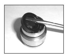
12. Use a flat screw driver to pry the oil seals (#19) loose from the seal case (#20).
