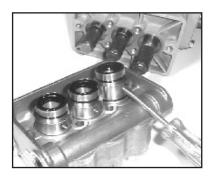
Remove weep return rings (#25) from the plungers (#16). Remove the seal case (#20) from either crankcases (#1) or manifold (#26) by using a screwdriver as shown above.
