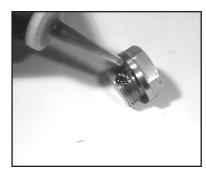
5. Apply one drop of Loctite 243 to valve plugs (32) and tighten to 59 ft.-lbs. For pumps manufactured prior to 5/97 tighten plugs to 37 ft-lbs.
