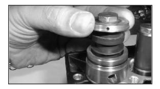
**15.** Place each seal case (#20) with o-rings (#21, 22) over the plungers (#16). Be certain the oil seal is centered with the seal case and tap firmly until the seal case is seated squarely on the crankcase (#1). Place pressure ring (#24) in seal case).
