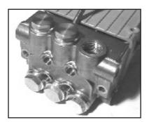
7. Carefully slide the valve casing (#26) out over the plungers with a screwdriver placed between the valve casing and crankcase.
