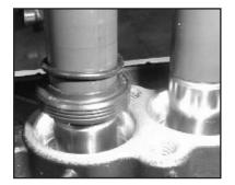
14. If the oil seals (#19) were removed, replace them with the primary seal lip (grooved side) towards the crankcase and the dust lip (tapered end) towards the valve casing (#26). Lubricate the seal before replacing. Install the oil scraper (#18) over the plunger.
