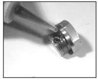
Apply one drop of Loctite 243 to the valve plugs (32) and tighten to 33 ft.-lbs.
