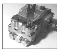
Using a needle nose pliers, remove the inlet and discharge valve assemblies (26A), for P230-5100 only, remove spacer (30A), and o-ring (31). Inspect all parts for wear and replace as necessary.
