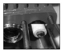
10) Check plunger surface (25 and 29B) for wear and pitting. If none is found, proceed to step twelve.
