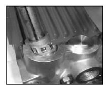
2) Remove discharge and inlet valve assemblies (46) by pulling them upwards out of the valve casing (43). It maybe necessary to use a slide hammer tool.
