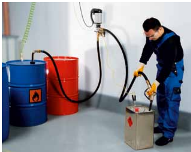
Filling of solvents from a 200 litre drum into different containers.
