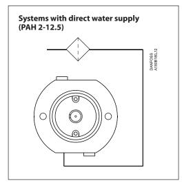
In order to eliminate the risk of cavitation, a positive inlet pressure is always to be maintained.
