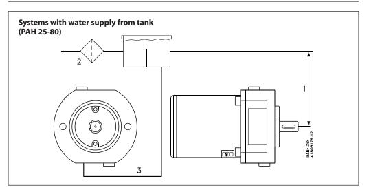
In order to eliminate the risk of cavitation, a positive inlet pressure should always be maintained by observing the following guidelines:
