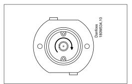
Clockwise (CW) seen from the pump shaft end (illustrated by a PAH 10/12.5).
