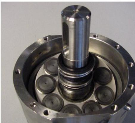
4. Wet the shaft and shaft seal with clean (filtered) soap-water.
