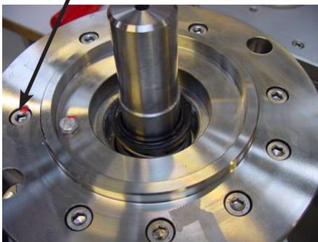
3. Carefully remove the flange from the casing.
