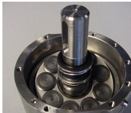
12. Remove the old O-ring and fit the new O-ring on the adapter.
