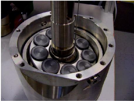
8. Fit the hollow bush (torpedo) onto the shaft.
