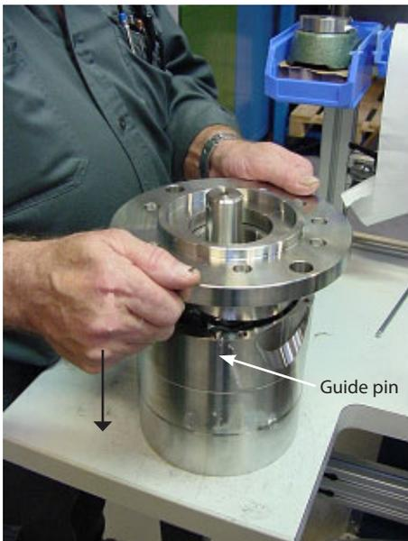
14. Screw the 8 screws into the flange and the casing. **To prevent cold welding, lubricate the threads on the 8 screws with grease**, screw them into the pump and tighten by hand. Use Molykote® D paste from Dow Corning or Klüber UH1 84-201 from Klüber Lubrication.
