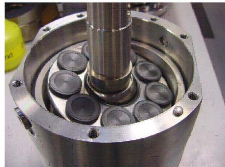
6. Ensure that no dirt has entered into the pump.
