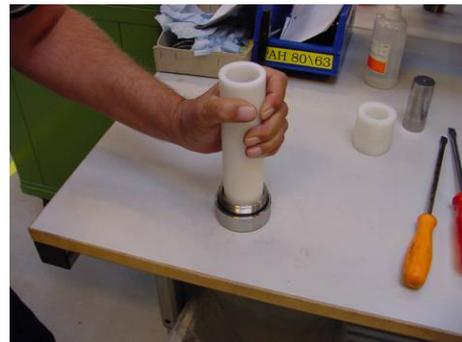
Make sure the face with the rubber seal is positioned against the shoulder in the retaining ring (see drawing on last page).
