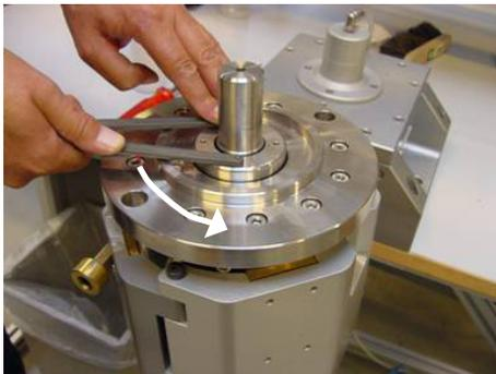
2. Unscrew the 8 screws in the mounting flange.
