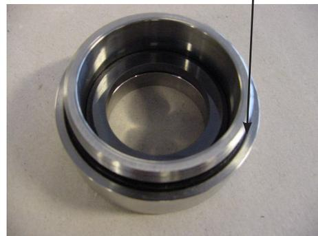
19. **To prevent cold welding, lubricate the thread and O-ring on the retaining ring with grease**, screw it into the pump and tighten it by hand.
