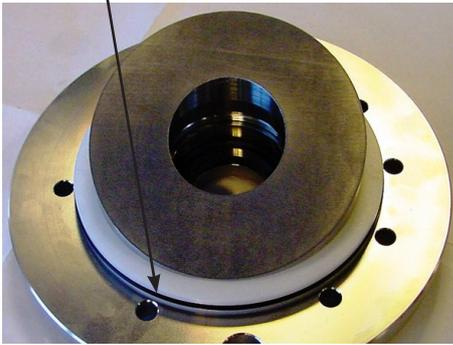
13. Place the guide pin in the casing. Position the combined flange and swash plate onto the guide pin and press it gently, by hand, into the casing.
