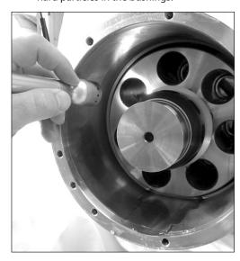
If any worn pistons are found, all pistons must be replaced. See page 7.
