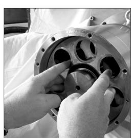
2. Ensure that the retainer plate is oriented correctly with its slant surfaces pointing downwards.
