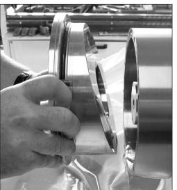
Mount the 3 screws as shown below. Turn each screw a couple of rounds at the time, to ensure the swash plate is pulled as straight forward as possible.
