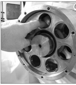
Inspect the piston bushings in the cylinder barrel for scratches or other damages.
