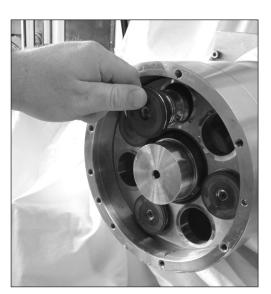
Note: Tilt the retainer plate for easy insert of the swash plate. Place pin in the housing.
