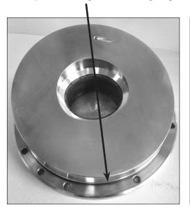
5. Carefully insert the swash plate into the housing.
