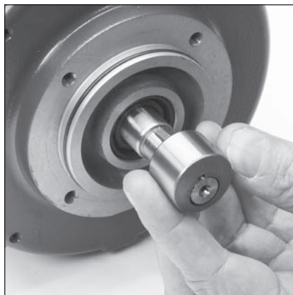
5.5 Remove and inspect cam (8) from motor shaft.
