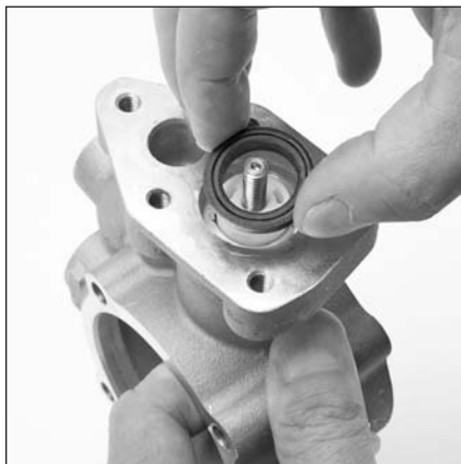
6.16 Lightly lubricate and install high pressure seal (22) with metal backing facing down over ceramic plunger (21).
