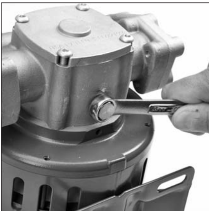
6.25 Install drain plug (3) into bottom port of crankcase body (1).
