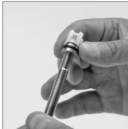
5.11 Thread M8 bolt so it makes contact with valve, continue threading until separation of retainer and seat.
