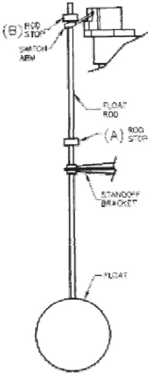
e. After setting all stops as described above, the sump should be filled with water. The pump should be checked for correct operation and desired ON/OFF water levels.
