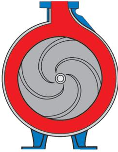
Both the **modified concentric volute** and **partial splitter** minimize radial loads and distribute pressure evenly across the entire flow range for less stress and wear on components. Casing meets ANSI B73.1 dimensional requirements for foot and flange.
