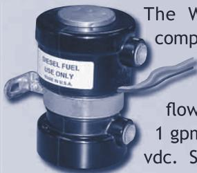
The Walbro electronic diesel fuel pump is UL listed, completely sealed and is supplied with a fully insulated double wire hookup. It utilizes a solenoid driven diaphragm to provide dependable suction and fluid flow for many applications. Each pump delivers up to 1 gpm, 7 psi, has 1/4" FPT ports and is available in 12 and 24 vdc. See page 47 for more information.
