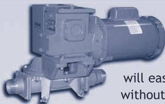
The diaphragm pumping principle is self-priming and will run dry indefinitely. Small and economical direct drive models will quickly lift bilge water up and force it overboard in short order. Larger sizes will easily pass solids that might pass through your strainer without clogging. Sizes are available that will deliver up to 20 gallons per minute. See page 39 for details.
