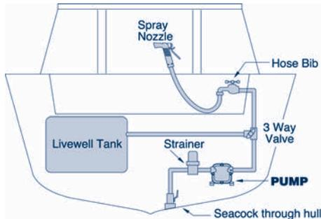
Washdown pumps come in two main varieties. High pressure, low flow models are typically self-priming and come with an automatic demand switch that controls their operation much like a water system pump. Low pressure, high flow models are operated by a manual switch and normally require flooded suction. Most washdown pumps can be utilized for baitwell operation. However, there are many models specifically designed for baitwell service.
