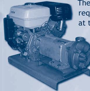
The owner of a water tanker truck had a request to deliver water to remote cabins at the top of a mountain. However, the closest he could maneuver his vehicle was 400' vertically below the highest cabin. He needed a solution. We recommended, assembled and sold this MTH turbine pump driven by a Honda gasoline engine.
