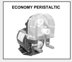
Need an economical peristaltic pump? Here is a 2.2 gpm, 1/4 hp, 115 vac model that will develop 20 psi and lift 15 feet! It even has a carrying handle! Can you beat that? (See page 47)
