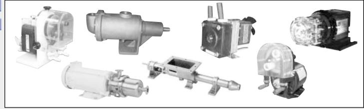
Progressive cavity and peristaltic pump types move a measured volume of material in a gentle, smooth fashion, and are able to handle solids and abrasives. Selection is limited by temperature and chemical compatibility of the hose on a peristaltic pump and the stator on a progressive cavity pump. (Sanitary models on page 102, precise metering models on page 120)
