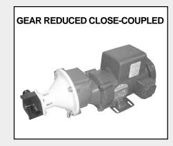
High viscosity? No problem! This epoxy flexible impeller pump has a 2 to 1 gear reducer to transfer a viscous liquid without any metal to liquid contact! (See pages 22-23).
