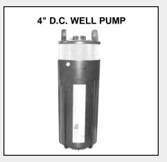
This 24 vdc solar or battery powered well supply pump will fit down a 4" well casing to a depth of 230' and supply water for a cabin, livestock, or a small irrigation system. (See page 131).
