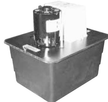
The reservoir on the March TCP-25 will hold up to 2 gallons! It pumps up to 100 gph, will lift up to 25', and will not airlock. It even has a hi-safety cut-off float switch. Now isn't that special! (See page 123)
