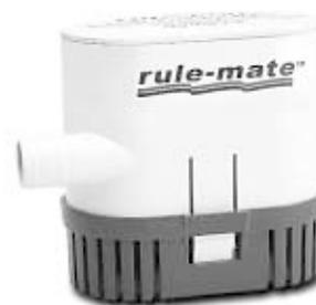
This is a low voltage DC (12 vdc) submersible pump with strainer and automatic controls. Its built-in float switch turns it on and a current sensor turns it off! (See page 128)
