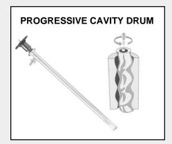
Need to get the 100,000 cps abrasive slurry out of your drum? This drum pump by Lutz will do the job! It's a progressive cavity drum pump that can be powered by electric or air. (See page 111).
