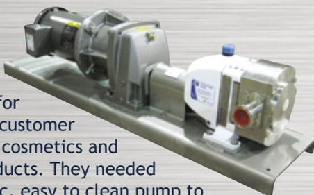
Problem: salad dressing transfer from several locations for a condiment manufacturer. The solution: a Jabsco sanitary "New Gen" 316SS flexible impeller pump, sanitary cart mounted to a 90 vdc/115 vac input variable speed control. This versatile pump can be used anywhere in the plant on many different products, cleans up very easily, is portable, and very economical to purchase and operate.
