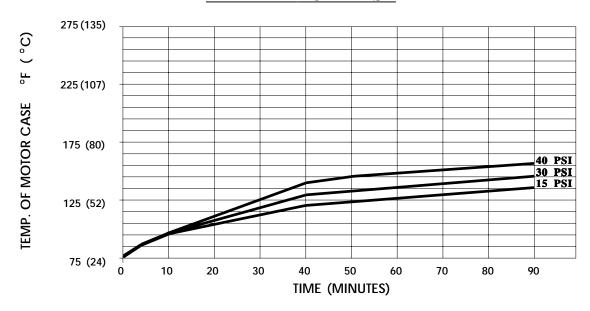
THIS GRAPH IS FOR USE AS A DESIGN GUIDE. IT IS BASED ON RUNNING CONTINUOUSLY WITH AN AMBIENT TEMPERATURE OF  $75^\circ$  F INSTILL AIR. THE THERMAL BREAKER WILL OPEN WHEN THE CASE TEMPERATURE REACHES  $280^\circ$  F.
