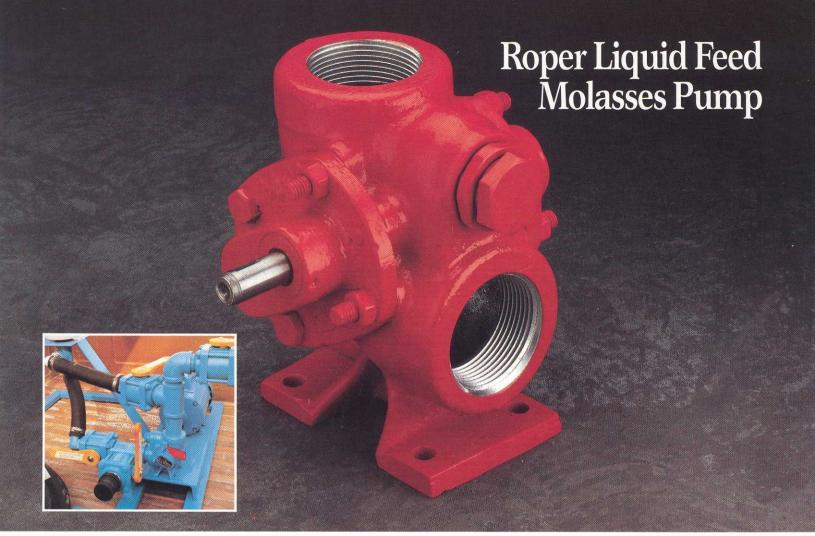
Roper's 2835 rotary pump is built for pumping highly viscous, molasses-based liquid feed supplements. The external helical gear design, combined with extra large ports, allows the 2835 pump to handle even winter-thickened feed supplements with ease. Highly viscous feed can be pumped at speeds of up to 1,800 RPM.
