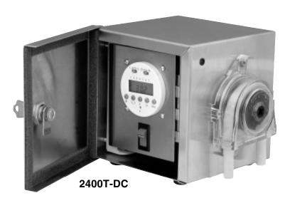
The new battery-powered 2400T-DC dispenser is designed for long battery life and is powered by easy-to-change, economical D-size batteries. A visual, low battery indicator is built in and the dispenser is housed in a lockable, stainless steel case. The programmable microprocessor features a 5-year lithium battery.
