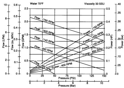
Notes: For continuous service: Plastic / Plastic gear combinations are limited to 50 psi. Metal / Plastic gear combinations are limited to 100 psi. Metal/Metal gear combinations are limited to 150 psi. Horsepower requirements increase for viscous fluids.
