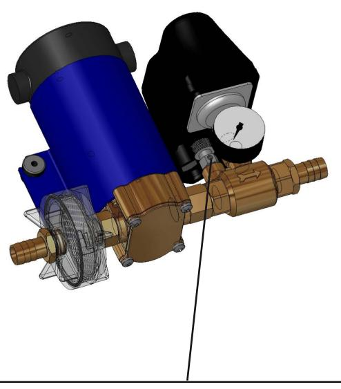
When starting the pump slightly open the small valve located next to the pressure switch, in order to let the air out and facilitate the pump priming. As soon as the pump is operating close the small valve.
