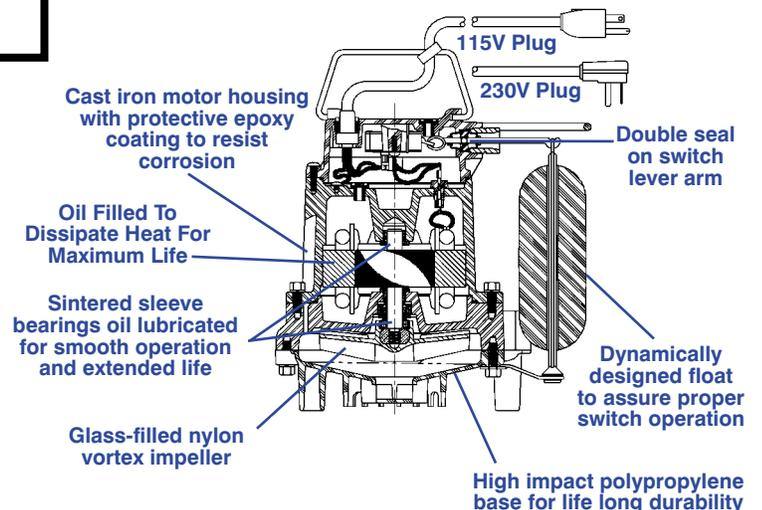
The model 6E Series Sump and Effluent Pumps are for residential and light commercial use. Pumps feature a 1-1/2" FNPT discharge with a lift of 20', polypropylene base and polycarbonate cover.
