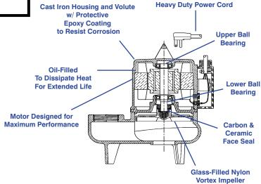
For increased pumping demands, the Model 10S Series Wastewater and Sewage Ejector pumps offer greater capacities than the 9S Series. Pumps feature a 2" discharge, with a lift of 20'. Cast iron housing and volute with protective epoxy coating.
