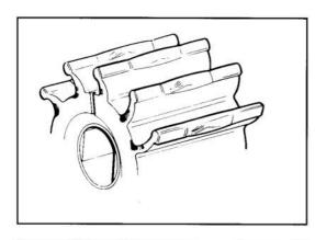
Symptoms: Worn blade tips, cam imprint on edges.
