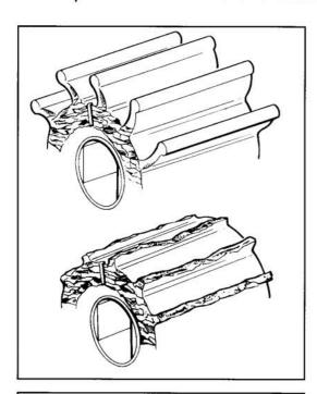
**Symptoms:** End faces hard and either polished or cracked.
