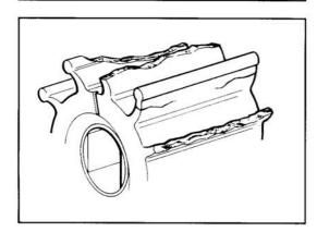
Symptoms: Blades cracked about half way up the length.
