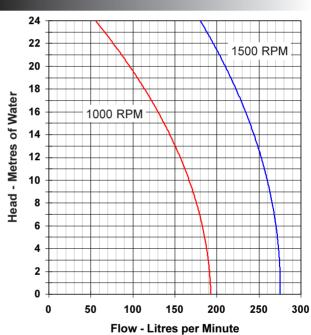
**Note**: Performance shown is for a new pump, fitted with a Neoprene impeller, pumping water at 20°C, performance may vary by up to 15%. Consult factory for performance of alternative impeller compounds.
