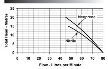
**Note**: Performance shown is for a new pump, pumping water at 20°C, performance may vary by up to 15%. Consult factory for performance of alternative impeller compounds.
