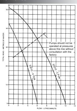
Note: Performance shown is for a new pump fitted with a Neoprene impeller pumping water at 20°C, performance may vary by up to 15%.
