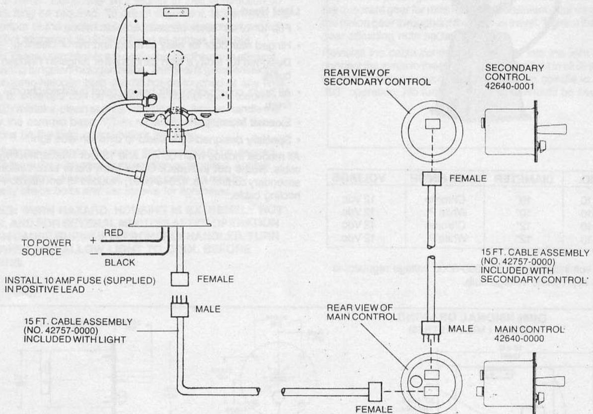
If additional cable is needed for main or secondary control connections, order 15 ft. cable assembly (No. 42757-0000) with mating plugs.
