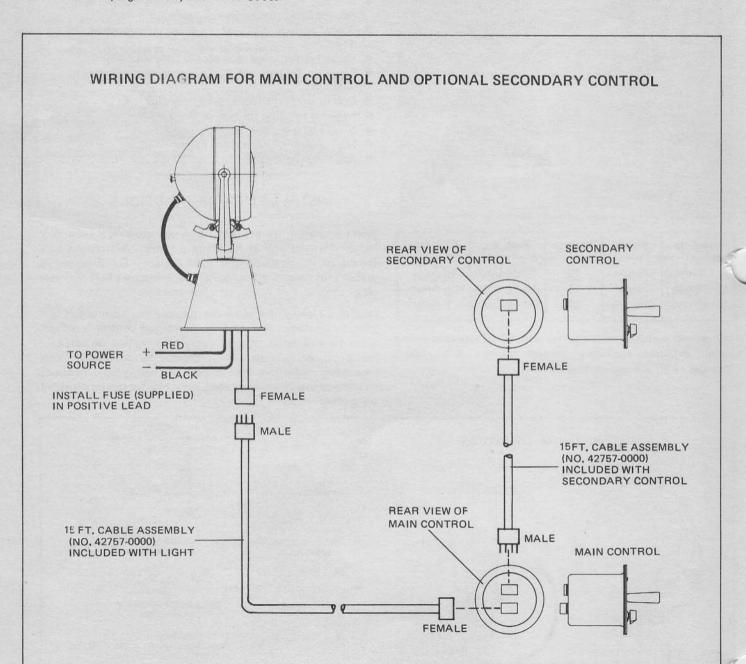
If additional cable is needed for main or secondary control connections, order 15 ft. cable assembly (no. 42757-0000) with mating plugs.
