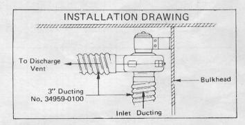
THE "WARNING" PLACARD SUPPLIED WITH BLOWER MUST BE MOUNTED ADJACENT TO ENGINE IGNITION SWITCHES (ALL LOCATIONS) TO COMPLY WITH TITLE 33, PART 183; SUBPART K, USCG VENTILATION REGULATIONS.\*
