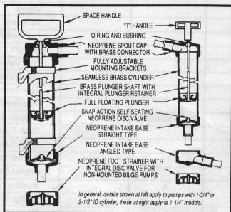
To reassemble pump, place disc valve in cylinder, snap intake cap back onto cylinder being sure undercut in cap is over cylinder roll. Insert plunger shaft assembly into cylinder and snap spout cap over cylinder roll.
