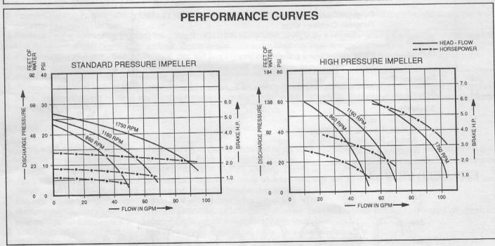
NOTE: Curves show approximate head flow for new pumps with neoprene impeller pumping water. Capacities should be reduced approximately 10% with nitrile and viton impellers.
