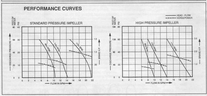
NOTE: Curves shows approximate head-flow for new pumps with neoprene impeller pumping water. Capacities should be reduced approximately 10% with nitrile and viton impellers.
