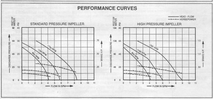
NOTE: Curves show approximate head flow for new pumps with neoprene impeller pumping water.
